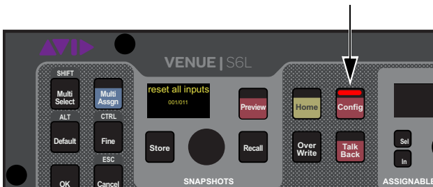
Config switch on the S6L control surface (left) and the Mode box showing Config
