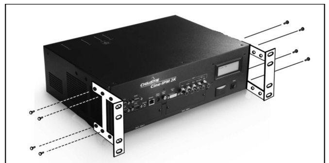
Figure 2.2. To Recess the Cine-IPM 2K
